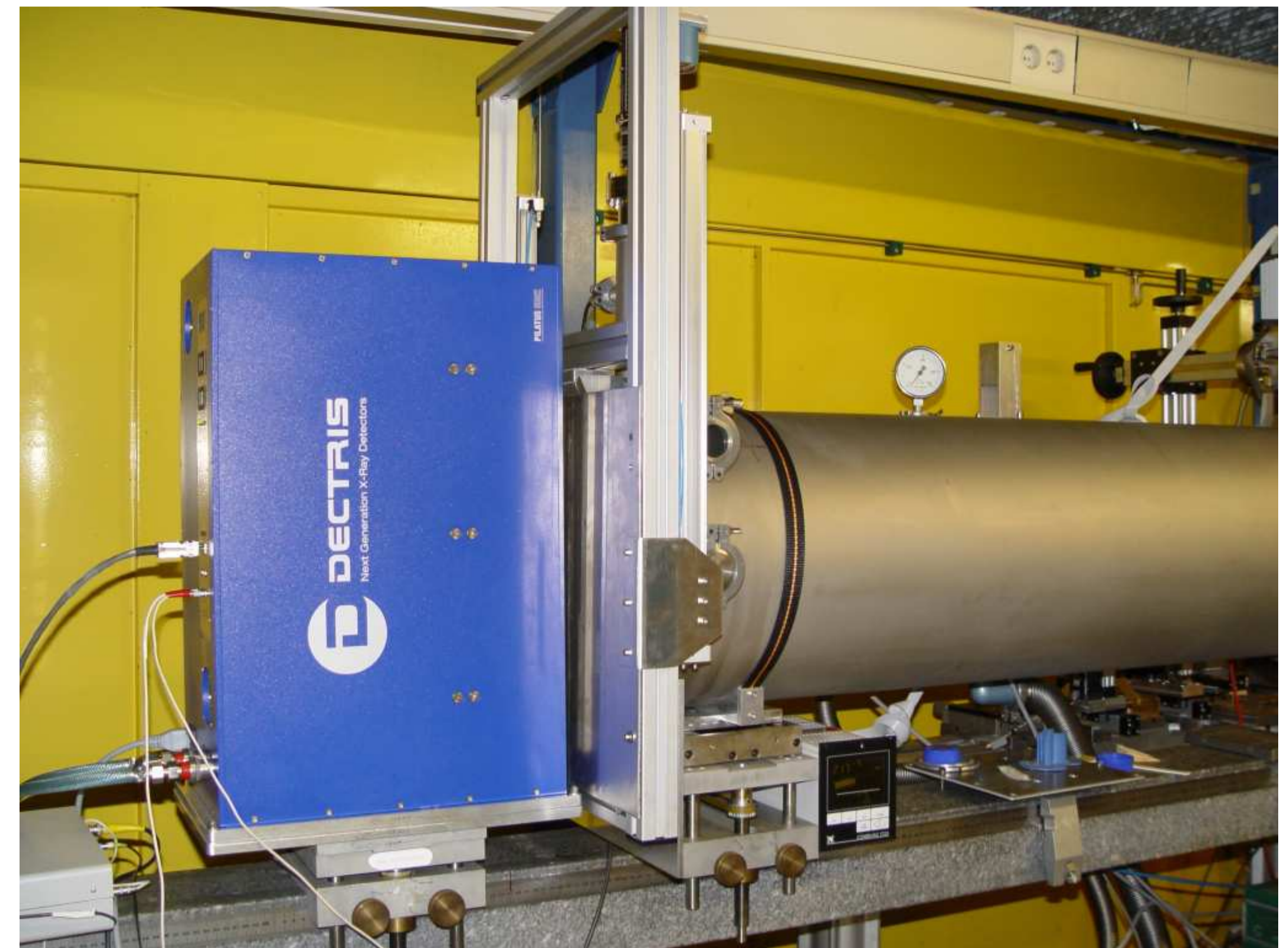
Figure 1: PILATUS 500k detector mounted at X33.
